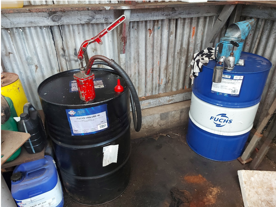
Photograph 3: Example of fuel/oil drums in the main workshop building. Note the staining on the ground surrounding the drums.
